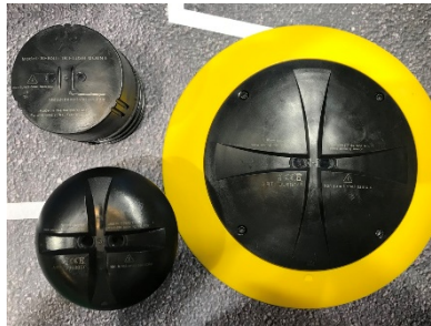
SENSIT parking sensor based on magnetic and infrared [2]
