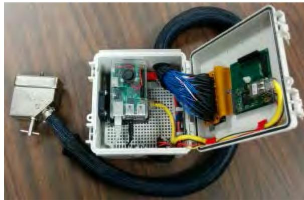
Electronic circuit: Samples all logic signals flowing in and out of a controller via a flex cable, makes individual contacts *with each C1 connector pin (104)*. Data is stored by a Raspberry Pi microcontroller, transmits to local USB thumb drive and/or web server program via TCP/IP.
