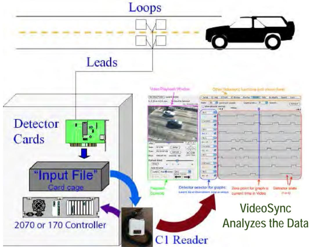
The C1 Reader collects the sensor data and transmits it to the VideoSync program.
